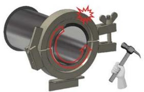
Longer pipes must be supported during the flanging process. The flanging tool is suitable for forming steel pipe ends with a material thickness of up to max. 2 mm. Welding ends should be used for pipe connections in case of a material thickness of 3 mm or more.
