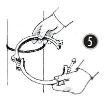
Open the clamping ring by rotating at the tension anchor. The entire clamping ring remains together as a unit including the screws.
