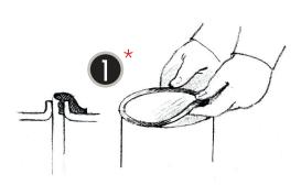
Select the seal ring according to the pipe diameter and pull it onto one of the lips. Start at the seam. The profiled side of the seal ring must face the connecting pipe. The seal ring may be drawn a little when pulling on.
