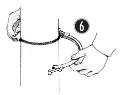
Place the clamping ring around the pipe parts and hook in the tension anchor.
