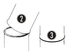
Place the connecting pipe evenly aligned onto the pipe with the fitted seal ring and check the fit.
