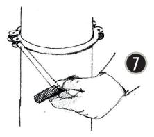
Finally, tighten both screws evenly with a torque of 10 Nm.
