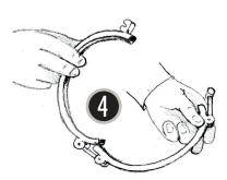
Loosen both clamping screws, but do not completely unscrew from the tension anchors. One of the tension anchors is gal-vanized yellow or, in the stainless steel version, has a groove. Unhook this tension anchor.
